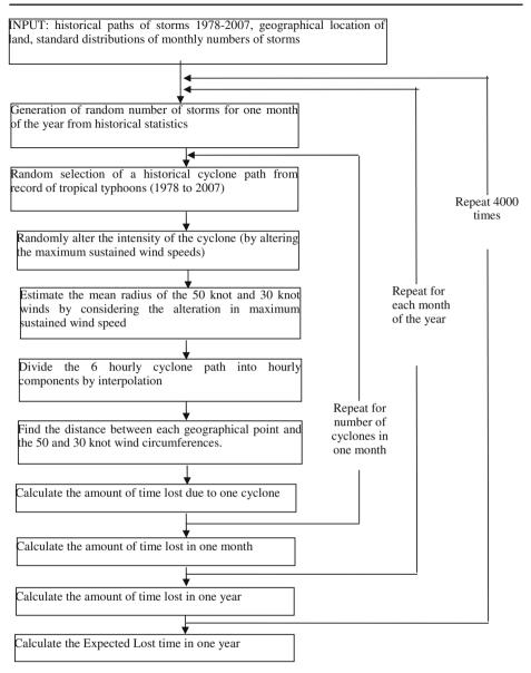
Fig. 1 Main loop of computation
