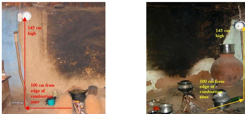
*Figure 5. Illustration of indoor air pollution instrument placement in homes. The horizontal measurement (100 cm) is made from the closest edge of the combustion zone and that the height is measured from the floor, not the top of the stove (145 cm).*
